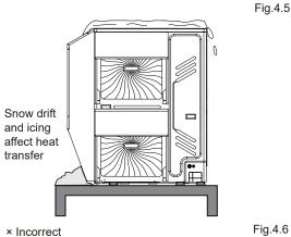
When multiple outdoor units are installed in severe cold areas, they should be arranged side by side. It is forbidden to stack two outdoor units up and down without protection to avoid icing of the outdoor units below.
