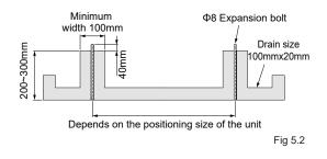
Use six bolts (M8) to secure the unit in place. Best is to screw in the ground bolt until it is embedded in the base surface by at least 3 threads.
