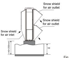
In severe cold areas, longitudinal foundation base shall be used to ensure that drainage is not obstructed. The height of foundation is recommended to be ≥ 500 mm.
