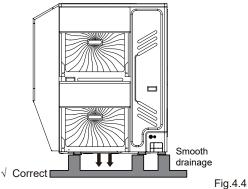
Avoid installation structure to clog the chassis drain holes, the mounting beam should be parallel to the unit to prevent the accumulation of ice and snow.
